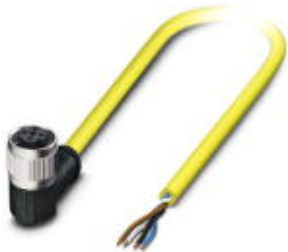
Sensor/Actuator cable, 4-position, PVC, Yellow RAL 1021, Free cable end, on Socket angled M12-SPEEDCON, A-coded, Cable length: 5 m
